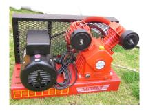
A small compressor will operate the pump. (An air tank or regulator is not required, but ok to have)
